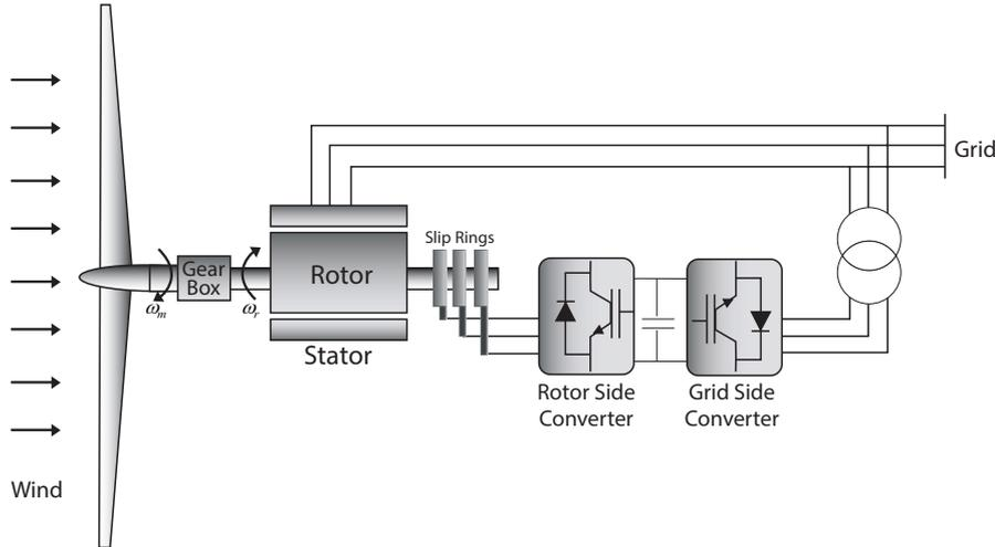
Fig. 1 Configuration of the DFIG wind turbine
