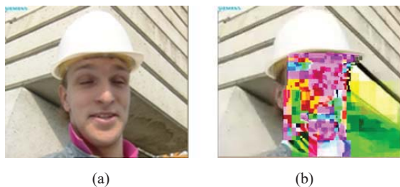
Fig. 4 Example for spatial drift due to change macroblock (a) original frame and (b) modified frame
