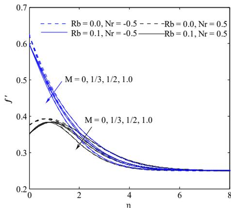
Fig. 23 Wedge angle parameter  $M$  effect on velocity distribution
