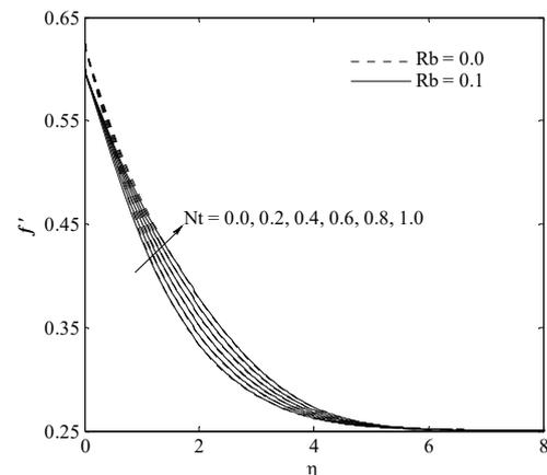
Fig. 7 Thermophoresis parameter  $Nt$  effect on velocity distribution
