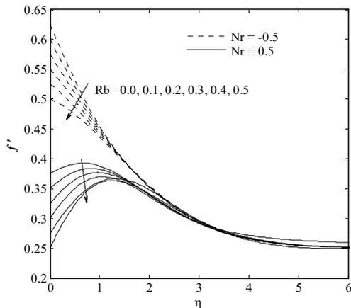
Fig. 5 Bioconvection Rayleigh number  $Rb$  effect on density velocity distribution
