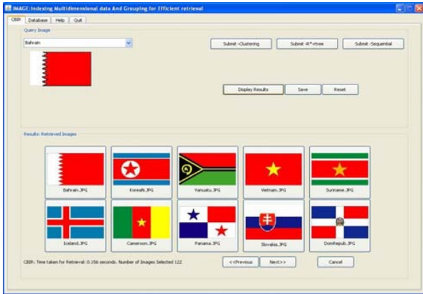
Fig. 7 Example of region-based image search using the representative color descriptor. The query is the red color of Bahrain flag
