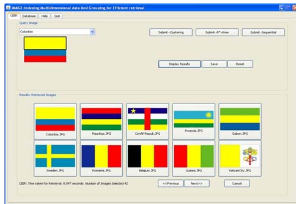
Fig. 6 Example of region-based image search using the representative color descriptor. The query is the yellow color of Columbia flag
