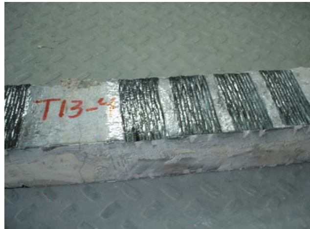
Fig. 7 Specimen prepared with grooving method
