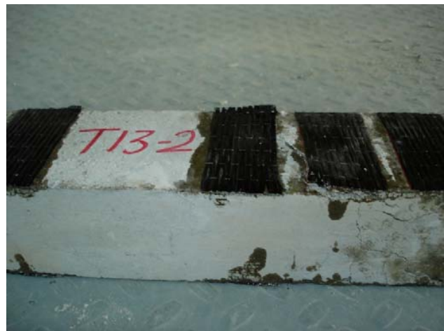
Fig. 6 Specimen prepared with surface preparation
