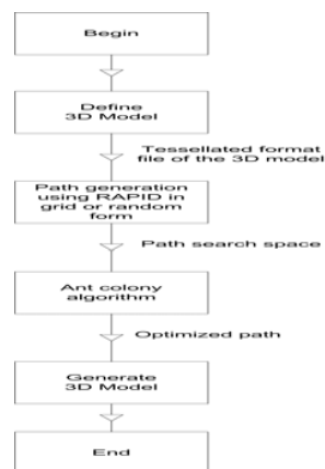
Fig. 1 Structure of the ant colony algorithm for automatic hose routing
