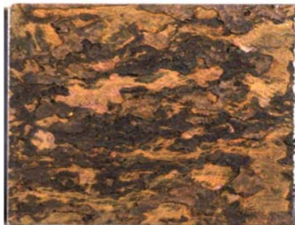
Fig. 7 Appearance of Corroded Surface before Painting (840 h SST, wire brushing)
