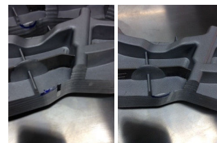
Fig. 2 Jig for tire production damage, holes, cracks meat parts (a) and jig for tire production, with thoughtful Image (b) [49]
