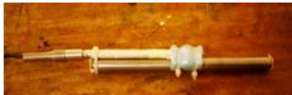
Fig. 2 Thermocouple J type, attached to the cylindrical probe
