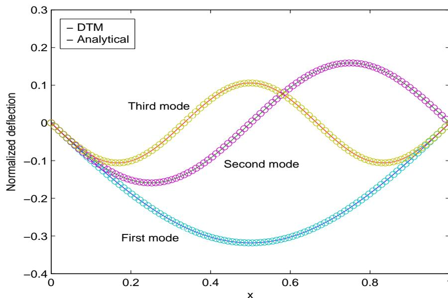
Fig. 1 First three mode shapes of homogenous beam
