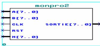
Fig. 10 Block of the Montgomery multiplication
