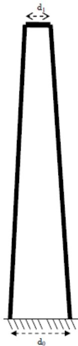
Fig. 3 (a) A geometrical model of a beam with large basis ( r < 1 )
