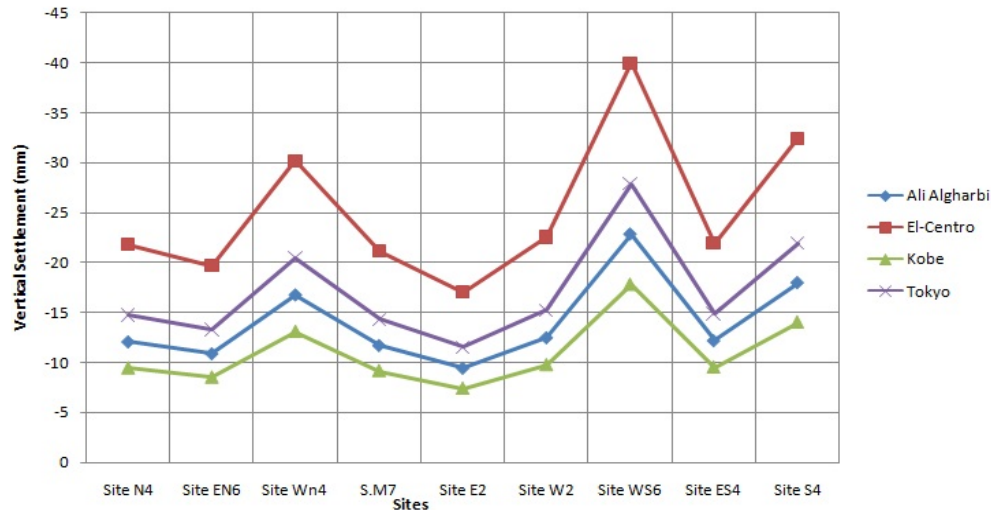
Fig. 11 Effect of different seismic waves on vertical settlement of raft foundation
