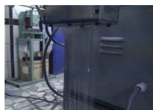
Fig. 2 Coat- Hanger die mounted on extruder and produced fibers [1]
