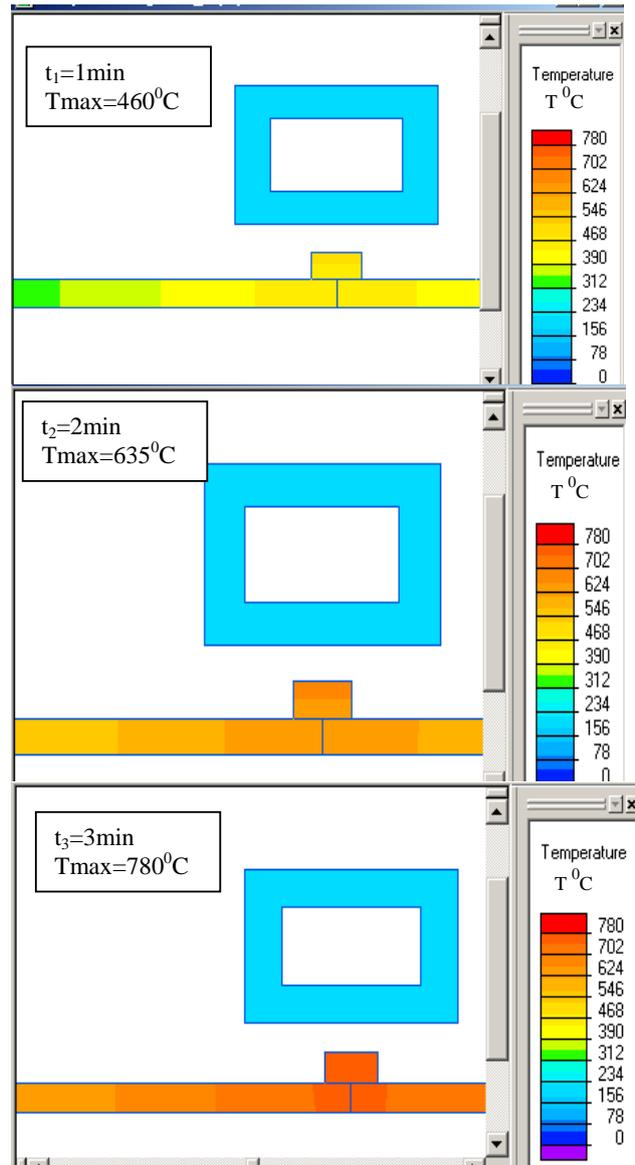
Fig. 6 Temperature change after 1, 2 and 3 minutes heating
