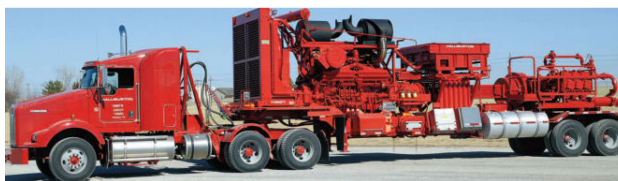
Fig. 1 Typical fracturing pump trailer
