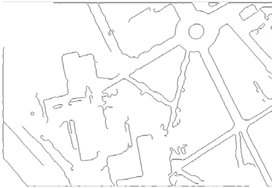
Fig. 2 Canny Operator Applied Image
