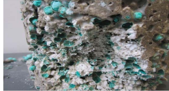
Fig. 2 Effect of alkaline environment on PLA aggregate
