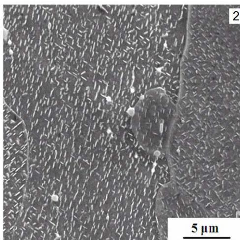
Fig. 3 Fine Fe<sub>16</sub>N<sub>2</sub> nitrides regularly dispersed in ferritic matrix
