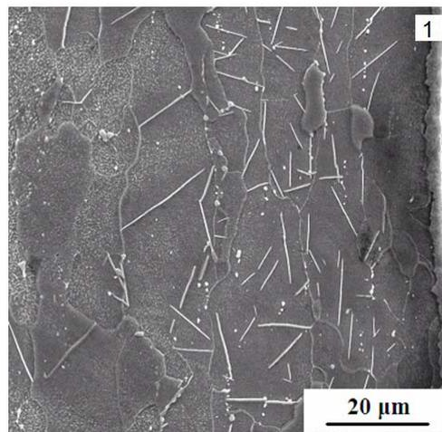
Fig. 2 Coarse needles of Fe<sub>4</sub>N nitrides
