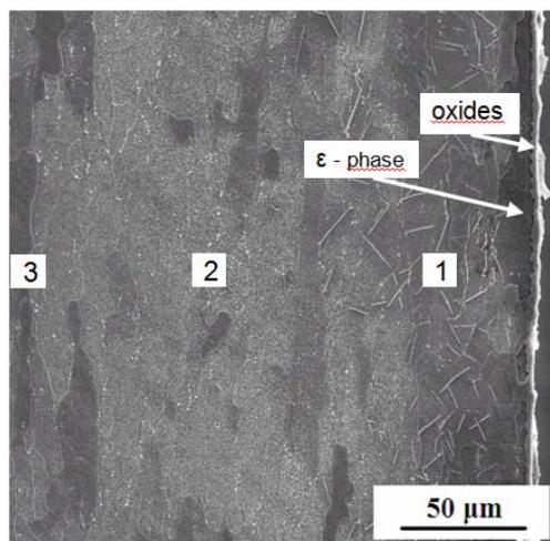
Fig. 1 Structure of DC 01 steel after nitrooxidation
