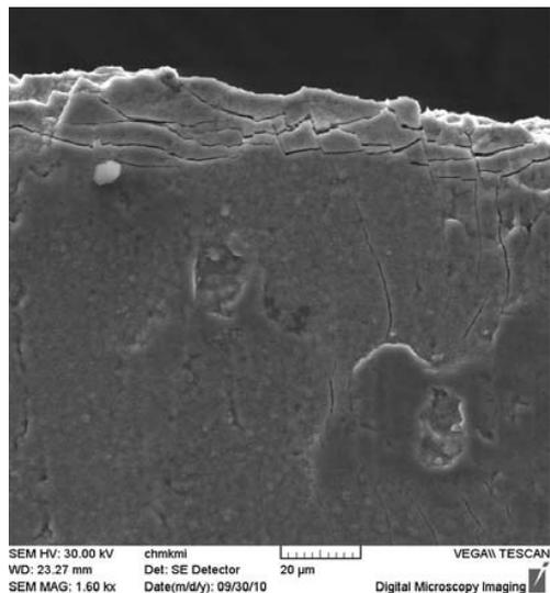
Fig. 10 Cracked nitridic layer at sheet surface in the place of fatigue crack initiation
