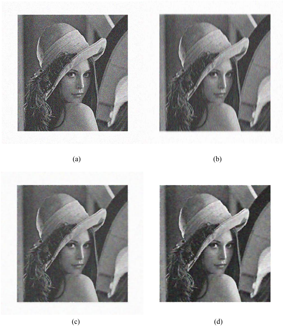
Fig. 7 Denoising results: (A) Lena image with additive Gaussian noise (MSE=285.72) (B) Wiener filter denoising (MSE= 58.83) (C) Wavelet thresholding (MSE=54.39) (D) Wavelet thresholding by local variance and edge analysis (MSE=53.51)
