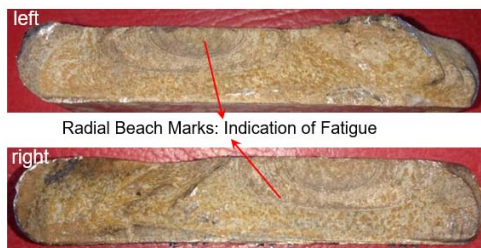
Fig. 2 Fracture surfaces at as-received condition
