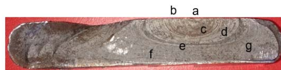
Fig. 6 Microscopic examination locations on the failed section
