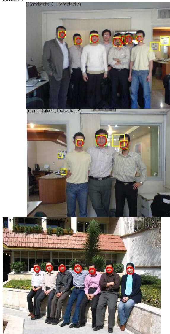
Fig.7 Some samples of obtained results (yellow rectangles: candidate faces by [15] and red circles: detected faces by our algorithm)
