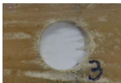
Fig. 4 Delaminated hole for hole 3
