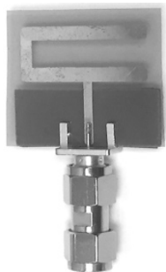
Fig. 2 The fabricated antenna using thermal deposition
