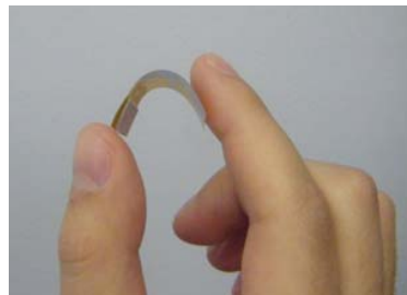
Fig. 1 Wearable inkjet-printed monopole antenna based on a Kapton Polyimide platform
