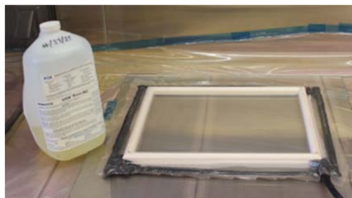
Fig. 1 Set up for preparation of core sheet
