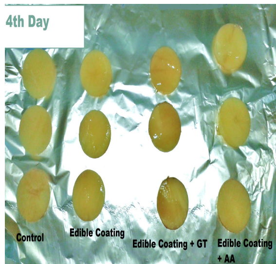
Fig. 2 Samples of potato slices after four days of storage in 4°C: a) control b) edible coating c) edible coating + GT d) edible coating + AA
