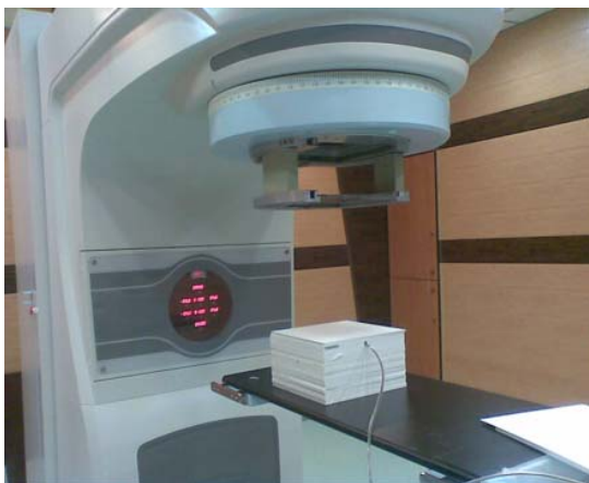
Fig. 2 set up for parallel-plate chamber measurements
