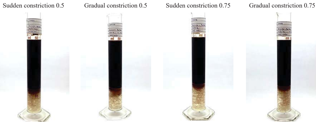
Fig. 10 Condition of 40 % crude oil after separation
