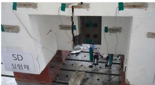
Fig. 8 Crack in SD Type
