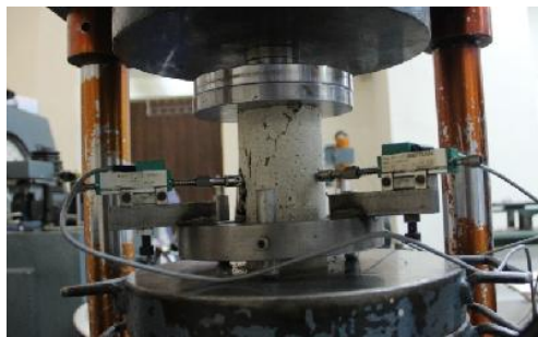
Fig. 3 Uniaxial compression test setup
