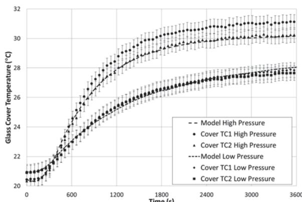
Fig. 5 Temperature of glass cover when passing 45°C water through the absorber plate
