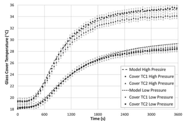
Fig. 6 Temperature of glass cover when passing 55°C water through the absorber plate
