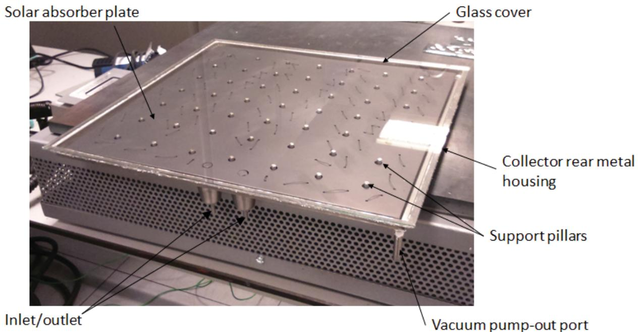
Fig. 4 Prototype of VFP solar thermal collector
