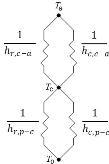
Fig. 3 Thermal-electrical analogy network for VFP collector.
