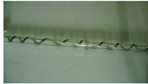
Fig. 2 Test section without insulation
