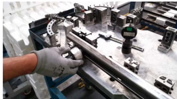
Fig. 8 Control of Roller Circulation Area between Master and Track
