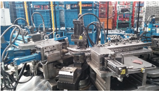
Fig. 6 Stretch Bending Operation
