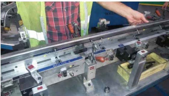
Fig. 10 Fixture Measured After the Stud Welding
