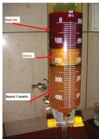
Fig. 1 Separated phases in the tower output sample
