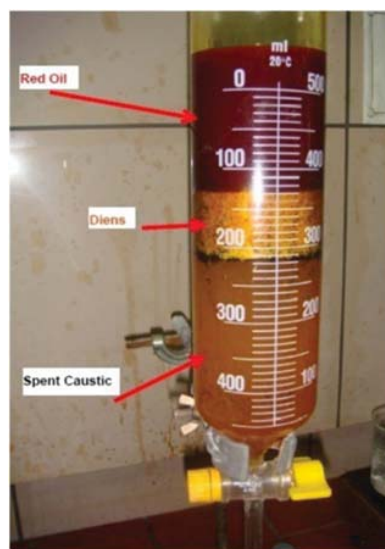
Fig. 1 Separated phases in the tower output sample
