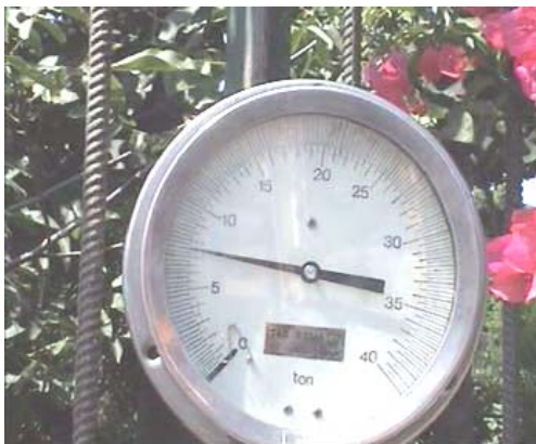
Fig. 5 Displaying the amount of force required to pull out the pile.
