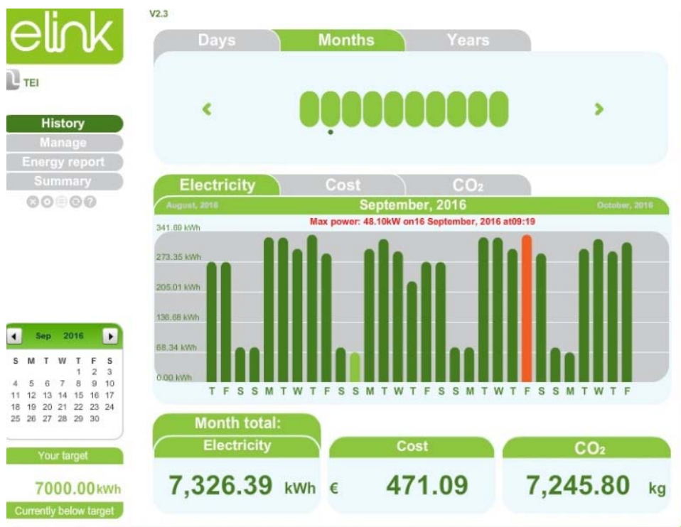
Fig. 4 Monthly electrical consumption of 2 nd power supply
