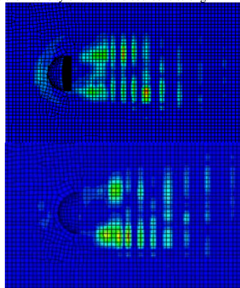
Fig.15 The dipole source on the mirror and plate surface returned by LES (up) and DES (down) (f=30Hz)
