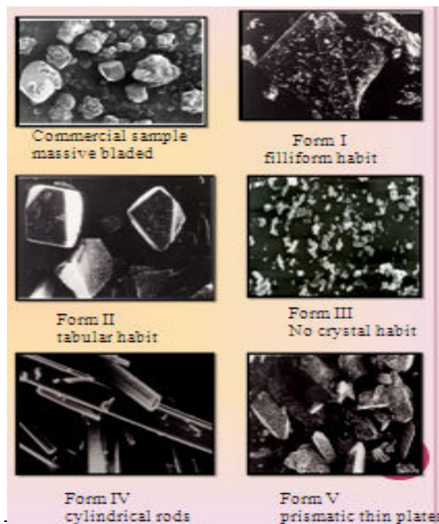
Fig. 1 Scanning electron micrographs of artesunate and its crystal modifications
