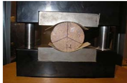
Fig. 3 Brazilian Test in laboratory
