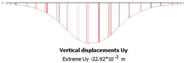
Fig. 16 The induced vertical displacement at the ground surface
