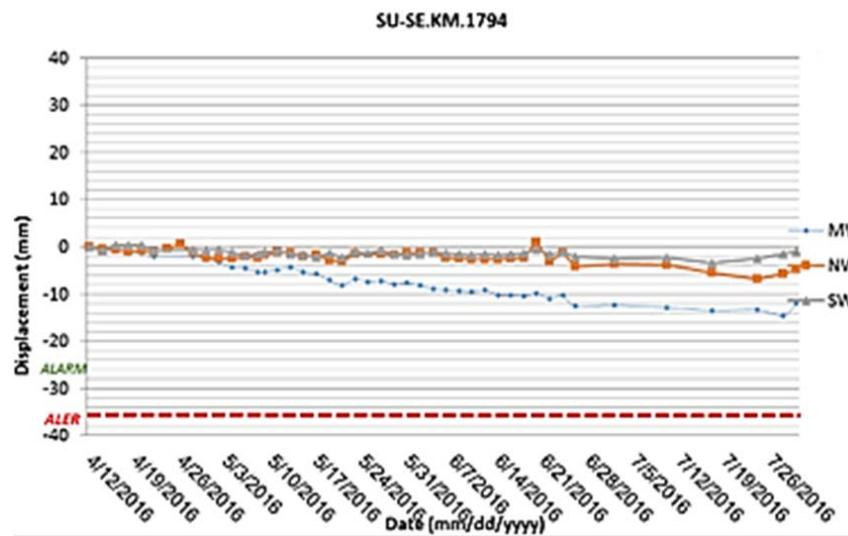
Fig. 10 The settlement readings of the top surface of the tunnel for three stages
