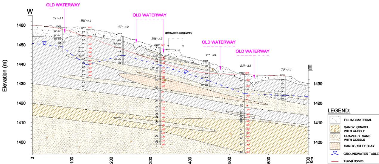
Fig. 8 Schematic geological layers of the project site
