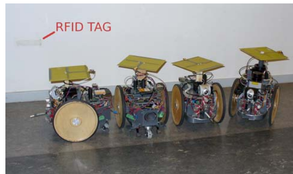
Fig. 5. Four MarsuBot robots used in the laboratory experiments. Directional RFID antenna on top of each robot. An RFID tag serving as a landmark can be seen on the background.
