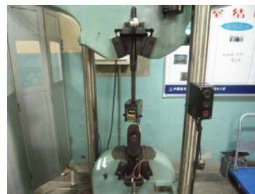
Fig. 6 Load test of the releasing device
