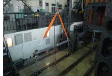
Fig. 7 Load test of single-beam hoist
