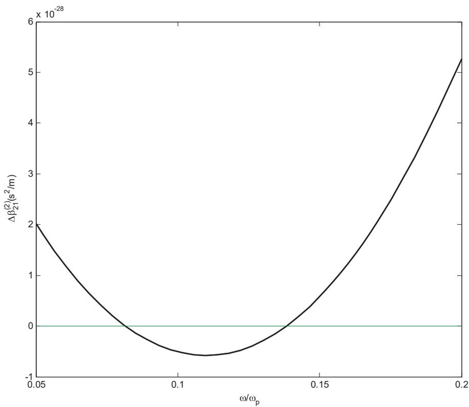
Fig. 7 Nonlinear second- order dispersion of  $\Delta\beta_{21}^{(2)}$  in three-layer structure of  $\text{As}_2\text{S}_3$  chalcogenide
