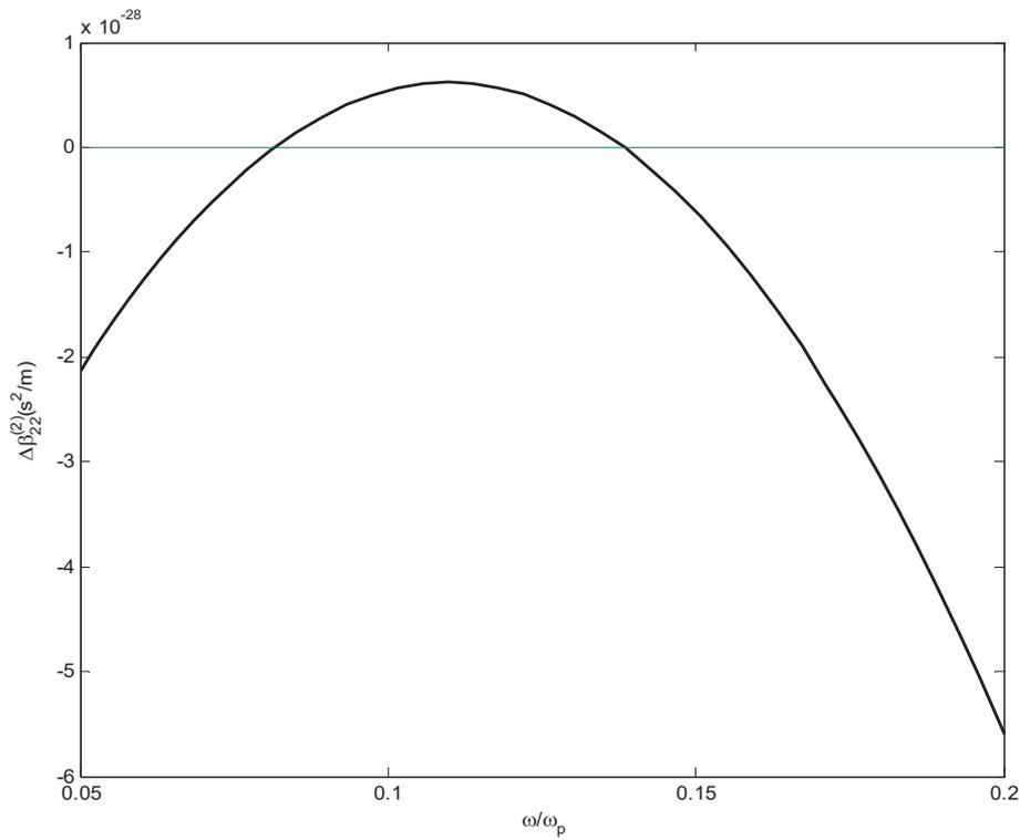
Fig. 6 Nonlinear second- order dispersion of  $\Delta\beta_{22}^{(2)}$  in three-layer structure of  $\text{As}_2\text{S}_3$  chalcogenide
