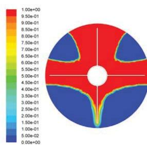
Fig. 3 (c) Melt Contour at 600 sec
