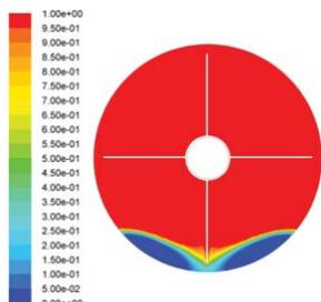
Fig. 3 (k) Melt Contour at 2200 sec
