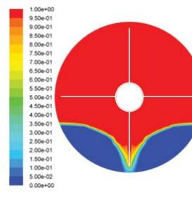
Fig. 3 (f) Melt Contour at 1200 sec
