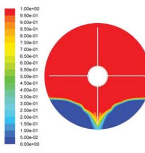
Fig. 3 (g) Melt Contour at 1400 sec
