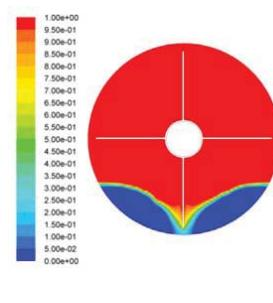
Fig. 3 (h) Melt Contour at 1600 sec
