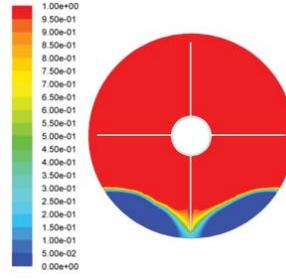
Fig. 3 (i) Melt Contour at 1800 sec
