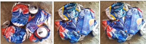
Fig. 12 Samples of real picture for the beverage cans after the densification process
