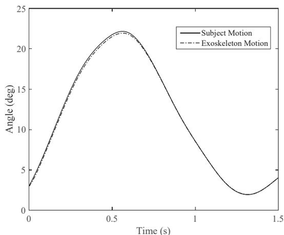
Fig. 10 Knee joint angle during leg swinging motion
