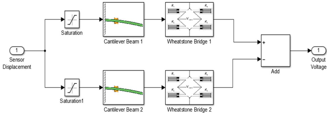
Fig. 8 Simulink model of the sensing subsystem
