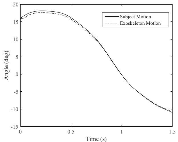
Fig. 9 Hip joint angle during leg swinging motion
