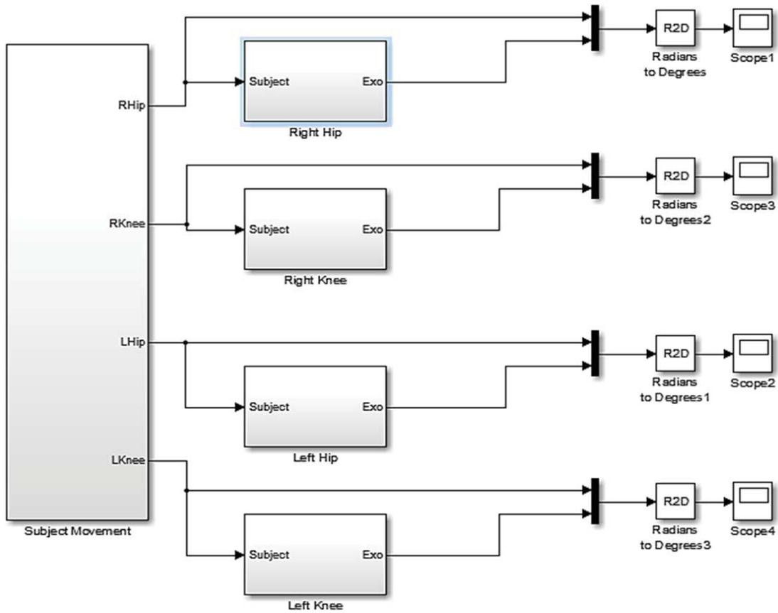
Fig. 5 Top layer of exoskeleton simulation program
