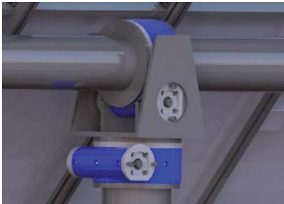
Fig. 11 Details of the drives in the final two axis solar tracker
