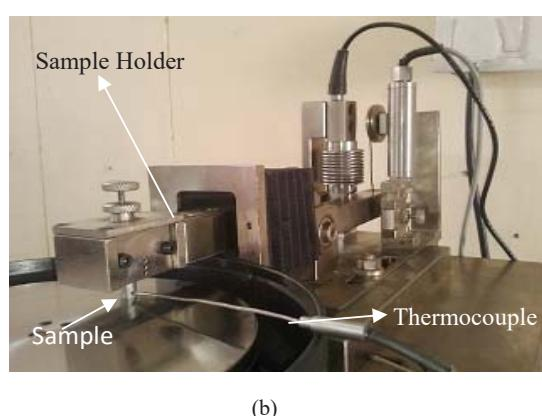
Fig. 1 (a) Schematic diagram of the wear testing machine (b) Magnified view of Pin-Disc Test Assembly
