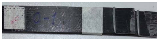
Fig. 4 The unidirectional adherents of single lap joint after the tensile test, which remained elastic without local or global failure
