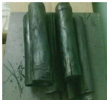
Fig. 4 Carbonized Bamboo Material
