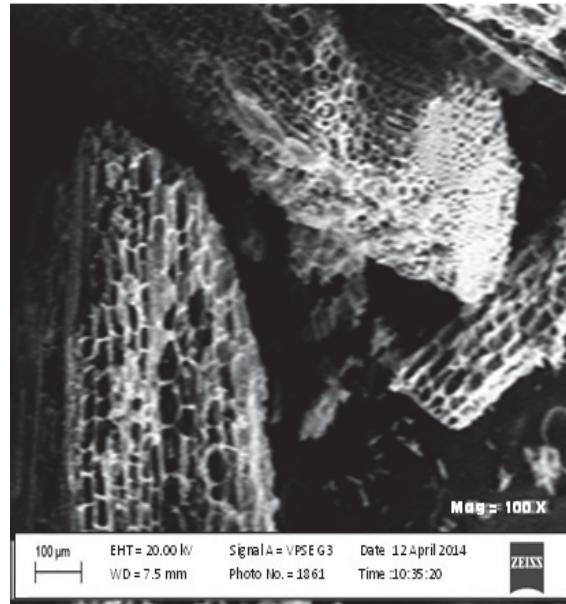
Fig. 7 Pore space of WBC at 20% ZnCl<sub>2</sub> Impregnation as viewed under SEM
