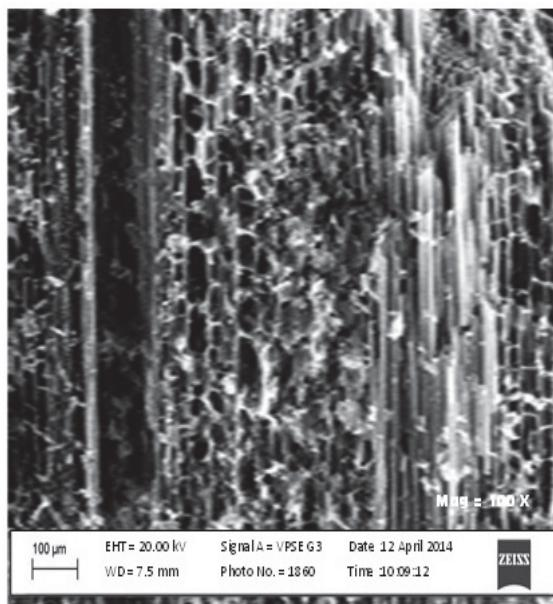
Fig. 5 Pore space of WBC at 0% ZnCl<sub>2</sub> Impregnation as viewed under SEM
