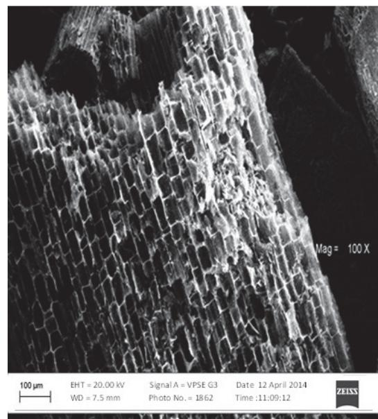
Fig. 6 Pore space of WBC at 10% ZnCl<sub>2</sub> Impregnation as viewed under SEM
