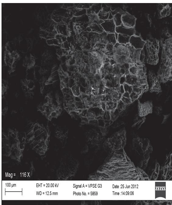
Fig. 10 Pore space of CPAC at 66%  $\text{ZnCl}_2$  Impregnation as viewed under SEM
