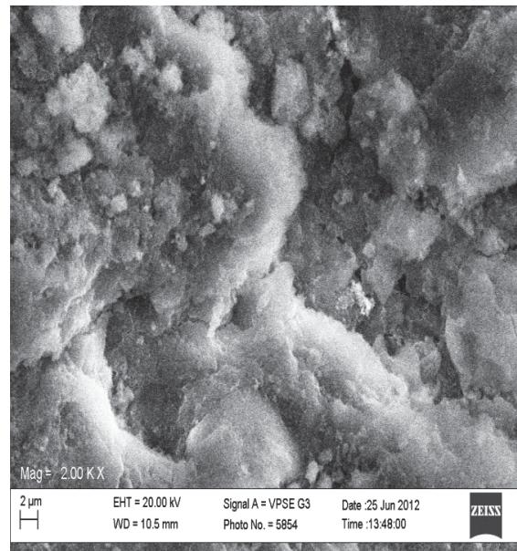
Fig. 8 Pore space of CPC at 0% ZnCl<sub>2</sub> Impregnation as viewed under SEM
